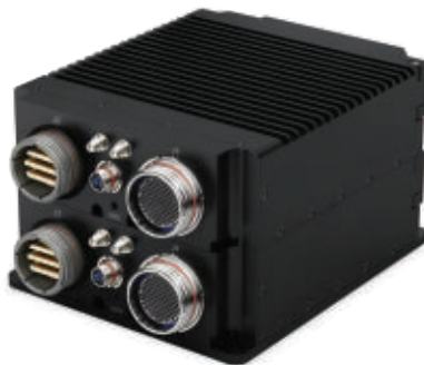
Mercury Systems uses special hardening to ruggedize high-performance embedded computing sufficiently for use in unmanned vehicle sensor-processing subsystems.
