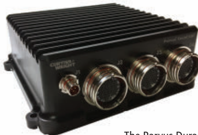
The Parvus DuraCOR 312 from Curtiss-Wright Defense Solutions is an ultra-small form factor embedded mission computer built around the NVIDIA Jetson Tegra X2 (TX2) integrated in a miniature rugged chassis with MIL-grade, high-density connectors.
