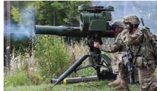
Operators control the TOW missile in flight using radio links between its launcher and the missile.
