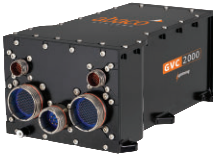
The GVC2000 from Abaco Systems is a mission or graphics computer intended for symbol generation, mission computing, demanding graphics generation applications, and GPU-accelerated data processing.
